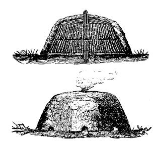
A setup for the manufacture of charcoal, pitch and tar
